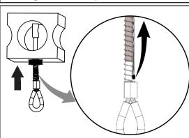
3. Push anchorage connector into drilled hole and engage toggle bar by pushing activator wire towards hole plug.
