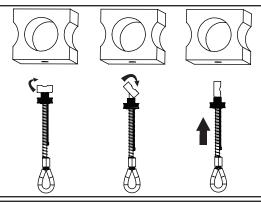
2. Rotate toggle bar into open position and insert into hole.
